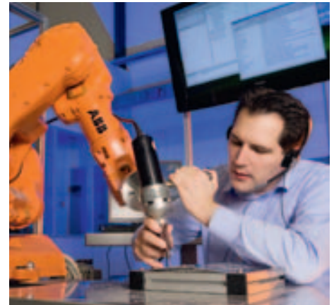
In "lead-through programming" robots are trained using hand and voice. The control software converts movements and spoken commands into a programme.
